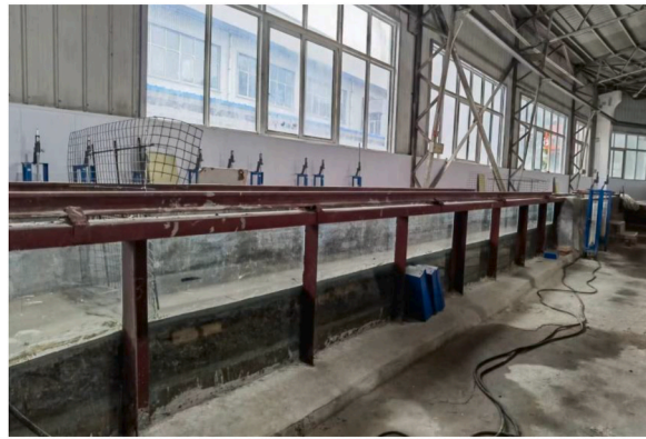
Fig. 2. A photograph of the test flume.
