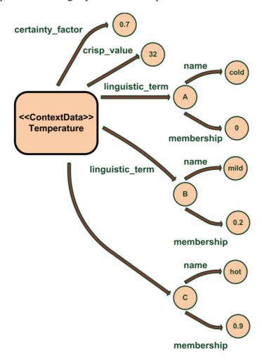
This can be seen in the example shown on Figure 2. The temperature measurement has a crisp value of 32 °C with a certainty factor of 0.7. After processing that crisp value with the associated membership functions our system has inferred that the membership degree for cold is 0, for mild is 0.2 and for hot is 0.9; so the room is mainly hot.
