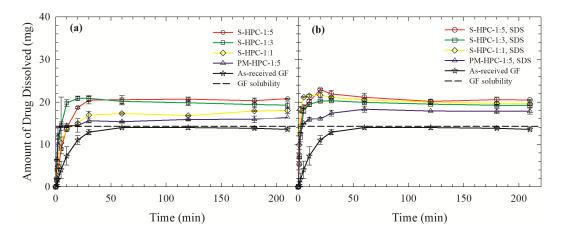
**Figure 5.** Evolution of drug release from as-received GF, physical mixture (PM) with a 1:5 GF:HPC mass ratio, and spray-dried powders prepared using the GF solutions with 1:1, 1:3, and 1:5 GF:HPC mass ratios: (a) HPC without SDS, (b) HPC with SDS.
