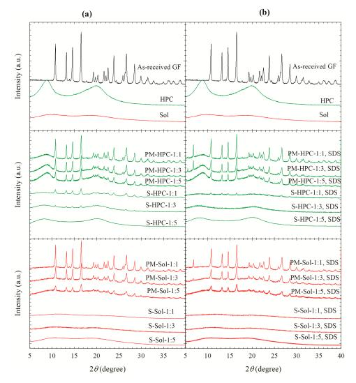
**Figure 2.** X-ray diffractograms of as-received GF, HPC, Sol, physical mixtures (PMs) of GF–HPC/Sol and the spray-dried powders prepared using the GF solutions with 1:1, 1:3, and 1:5 drug:polymer mass ratios: (a) without SDS and (b) with 0.125% SDS.
