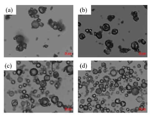
**Figure 1.** Light microscope images of the spray-dried particles prepared using the GF solution with a 1:3 GF:polymer mass ratio and 0.125% SDS/without SDS: (a) S-HPC-1:3, (b) S-HPC-1:3, SDS, (c) S-Sol-1:3, and (d) S-Sol-1:3, SDS. All images were taken at  $50 \times$  magnification (scale bar: 20  $\mu$ m).
