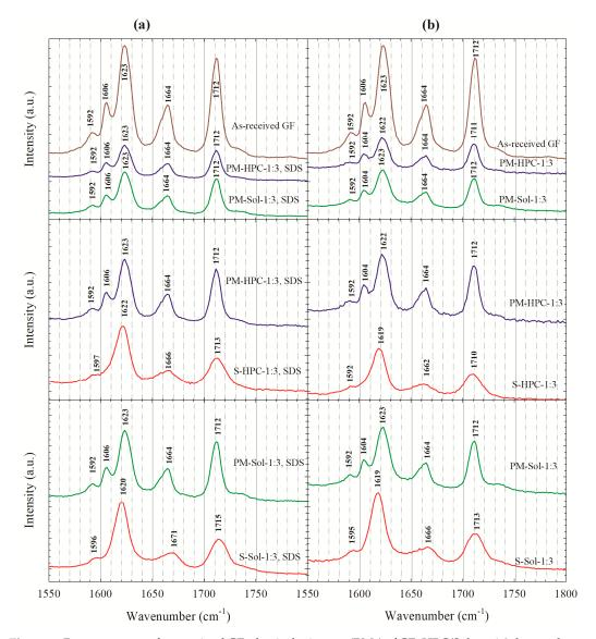
**Figure 4.** Raman spectra of as-received GF, physical mixtures (PMs) of GF–HPC/Sol at a 1:3 drug:polymer ratio, and the spray-dried powders prepared using the GF solution with a 1:3 GF:polymer mass ratio: (a) with 0.125% SDS and (b) without SDS.
