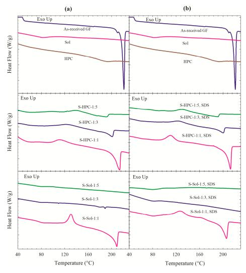
**Figure 3.** DSC traces of as-received GF, HPC, Sol, and the spray-dried powders prepared using the GF solutions with 1:1, 1:3, and 1:5 drug:polymer mass ratios: (a) without SDS and (b) with 0.125% SDS.
