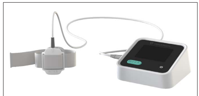
Figure 1. Picture rendering of the non-invasive venous waveform analysis (NIVA) device. The NIVA device is composed of a wristband used to capture the venous waveforms using a piezoelectric sensor encased in Versaflex as well as a main device where the signal is amplified and digitally processed on a microcontroller. The measured venous waveform contains the cardiac and respiratory harmonics in coronavirus disease 2019 and control subjects.
