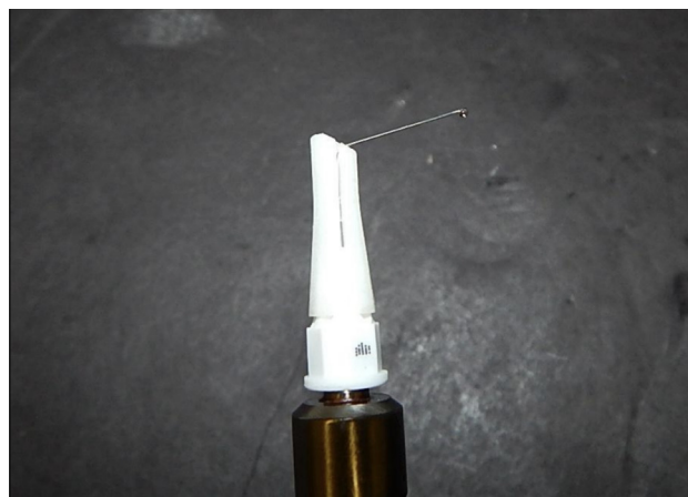
Fig. 1. Photograph of a needle bend using a needle guide.
