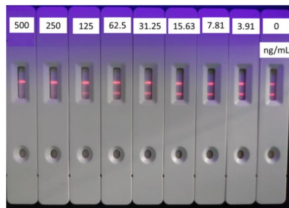
Figure 6. Standard curve for tylosin with coating antigen of 0.25 mg/mL ( n = 3 ). (The concentration of second antibody is 0.093 mg/mL.)
