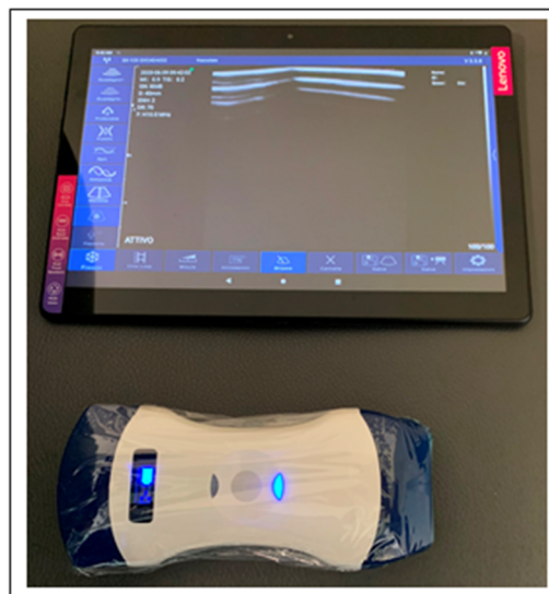
Figure 2. Wireless ultrasound equipment to avoid contamination. A wireless ultrasound probe with respectively a 4.5 mHz convex probe on the right side, and a 7.5 mHz linear probe on the left one. The transducer, wrapped with a single use plastic cover to avoid contamination, is wi-fi connected with the tablet which in turn, is encircled by a plastic film.
