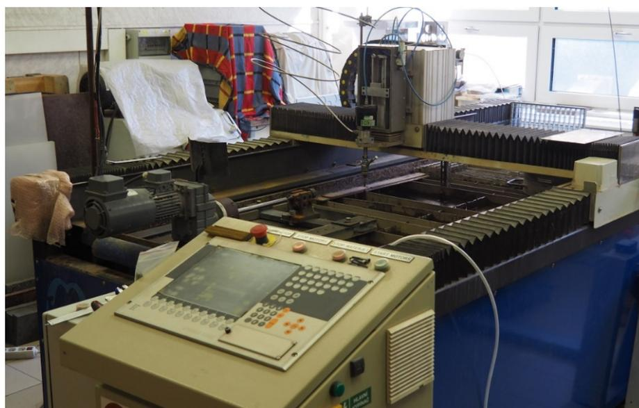
**Figure 2.** Abrasive waterjet laboratory with PTV WJ1020-1Z-EKO device.
