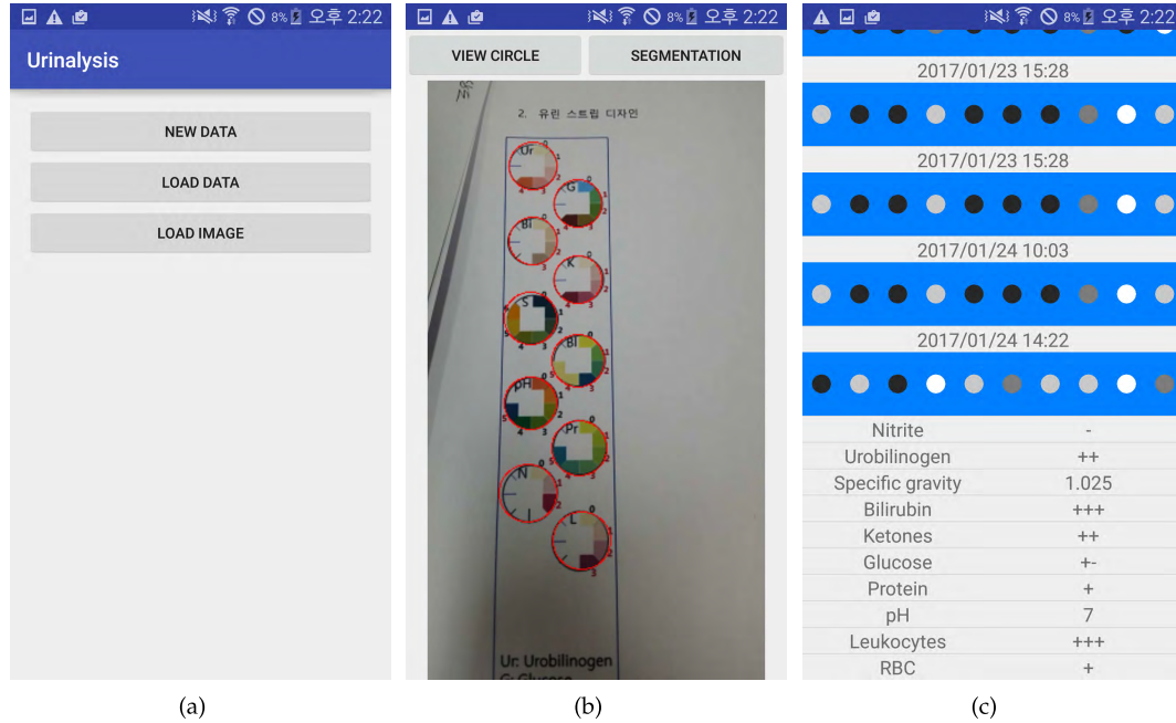
FIGURE 3. Developed smart-phone application for Android software using the proposed method. (a) Loading new data. (b) Detecting the strip for urinalysis. (c) Displaying results.
