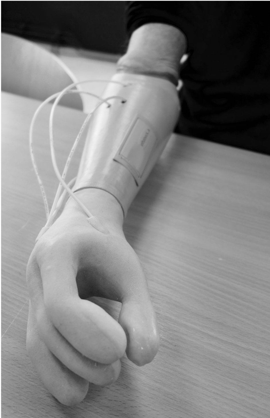
FIGURE 1 | When the silicon bulbs in the fingertips were pressed, the air was transferred via plastic tubes that reached actuators inside the prosthetic socket and gave pressure (mechanotactile feedback) on the skin corresponding with the PHM zones.
