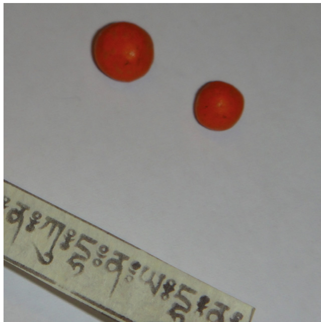
Figure 1. The analysis of the two pellets (0.5–1 cm Ø) showed the presence of a high level of lead on the surrounding red paint.
