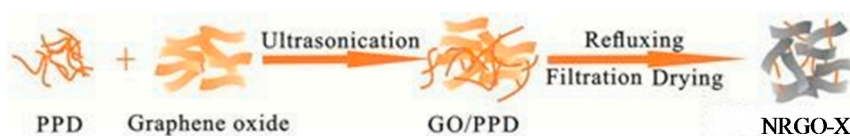
Figure 1. The preparation process of the PPD nitrogen-doped reduced graphene oxide.
