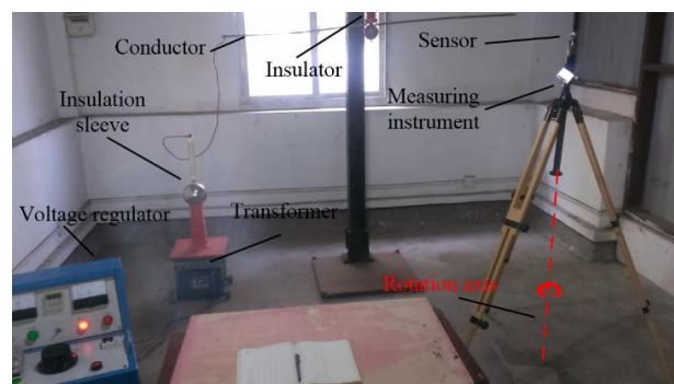
Figure 11. Experiment for testing the directional characteristic of the sensor.
