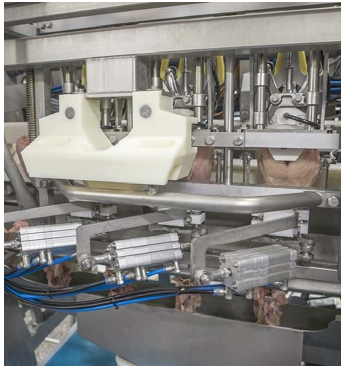
Figure 3. A new generation of automatic breast fillet deboning with the capabilities of measuring the size of each bone-in breast fillet portion to allow adaptive filleting of different size birds. The new generation machines also allow producing a range of products such as half fillets with/without skin, butterfly with/without tenders. Photo courtesy of Marel.
