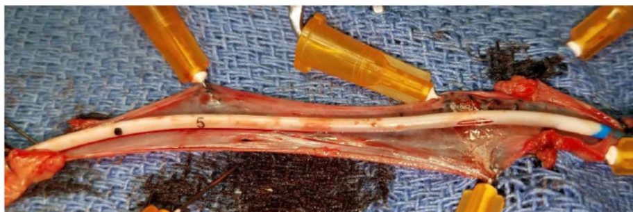
Figure 10. A NO releasing central venous catheter (CVC) with mounted electrochemical lactate sensor after 10 h of placement within a femoral vein during the in vivo porcine study. The catheter orifice provides a measurement window for the active sensing region.
