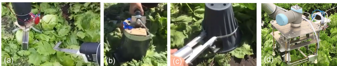
FIGURE 7 Development of lettuce harvesting end effectors. (a) Two-handed approach with one hand to hold the lettuce, one hand with knife, (b) rotary DC motor cutting mechanisms, (c) linear actuator knife-powered mechanism, and (d) pneumatic cutter chosen as the best mechanism [Color figure can be viewed at wileyonlinelibrary.com ]
