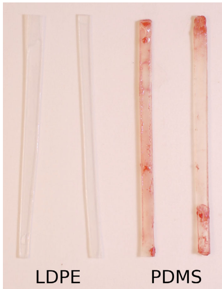
FIGURE 2. Macroscopic image of low-density polyethylene (LDPE) and polydimethylsiloxane (PDMS) flat sheets after in vitro incubation under pulsatile flow with physiological wall shear stress conditions with human whole blood at 37°C for 1 h. LDPE barely showing thrombus formation; PDMS clearly showing vast red-thrombus formation.
