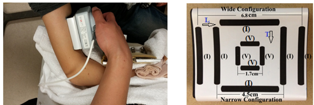
Fig 1. Position of the probe and a close up of the handheld electrode array configurations. (I) means current electrodes; (V) means voltage electrodes; L with arrow means the longitudinal direction; T with arrow means the transverse direction.
