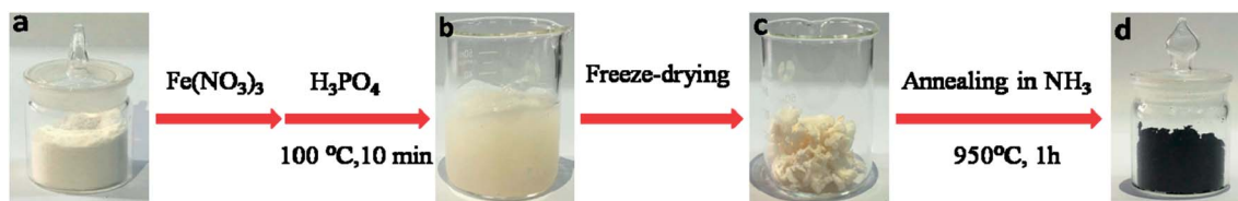
Scheme 1 Illustration of the typical N,P,Fe-NPC preparation. Photographs of Pueraria lobata powder (a), Pueraria lobata gel containing \text{H}_3\text{PO}_4 and \text{Fe}(\text{NO}_3)_3 \cdot 9\text{H}_2\text{O} (b), the material precursor obtained from the gel (c), and typical N,P,Fe-NPC (d).
