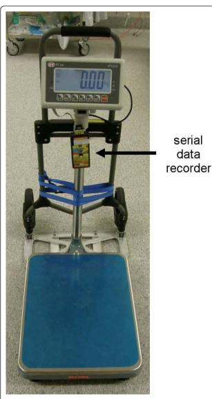
Figure 1 Platform scale with pole mounted display and serial data logger connected, secured to a hand trolley.
