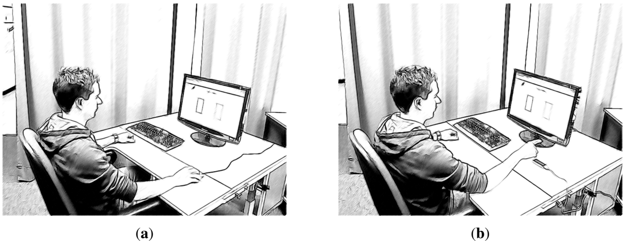
Figure 2. Experimental set-up: (a) participant using the mouse controller and (b) utilizing the Leap Motion Controller (LMC) to perform selection tasks.
