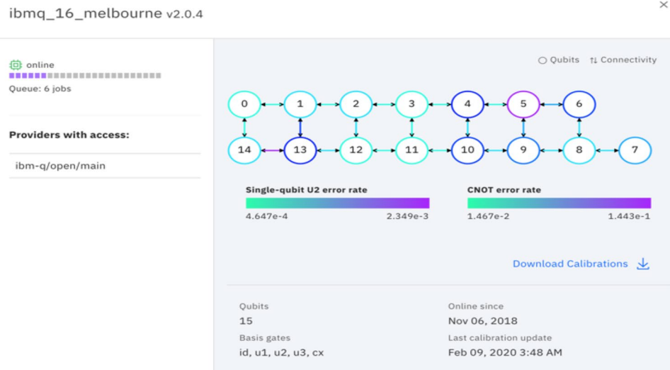
Figure 8. A diagram of single- and multi-qubit error rates in ibmq_16_melbourne , provided by IBMQ.
