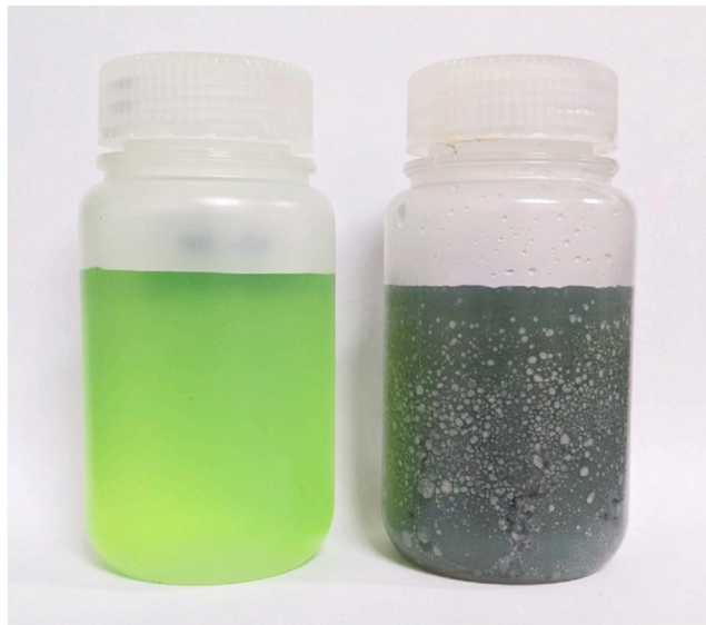
Figure 5. Photograph of a freshly prepared ELD Ni solution (left) next to a solution that has plated out (right)
