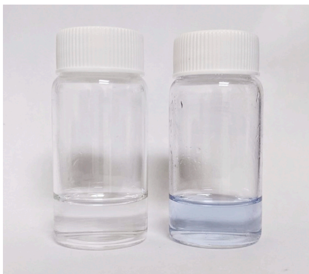
Figure 2. Photograph of a freshly prepared immersion gold solution (left) next to a depleted immersion gold solution (right)
