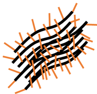
Figure 13. Aggregation of the APE r.ch. -graft-PiPrOx macromolecules in water.
