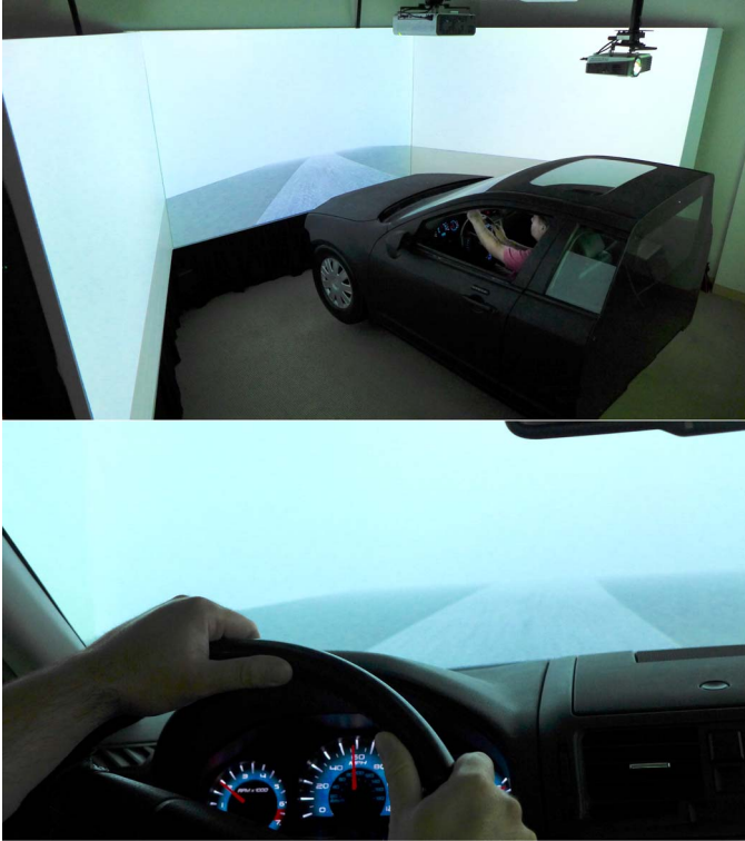
Figure 2. Curve negotiation task under fog condition. The task required drivers to drive on an ordinary winding road within a lane width of 3.6 m with a fog that limited preview to 30 m.
