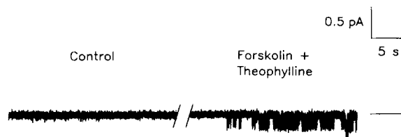
FIGURE 5. Activation of Cl - channels in the apical membrane of intact epithelium by cAMP. Cell-attached patch held at V_p = 0 mV. Zero-current levels are indicated to the right of the records. The record on the right starts 80 s after addition of forskolin plus theophylline to the apical bathing solution. In three experiments, single-channel currents were evident within ~3 min of drug addition. Pipette, NaCl solution; bath, NaCl-PSS; both were buffered with HEPES (pH 7.40).
