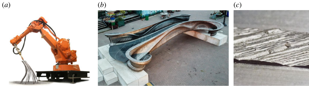
Figure 1. (a) The three-dimensional printing protocol developed by MX3D uses a weld head attached to a robotic arm (image by Joris Laarman, www.jorislaarman.com ). (b) Pedestrian bridge manufactured using three-dimensional-printed steel [5]. (c) Close-up of the geometric variation on the surface of the material [6]. (Online version in colour.)
