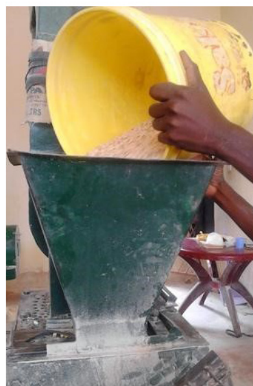
Figure 1. “Posho” mill grinding legumes to create flour.
