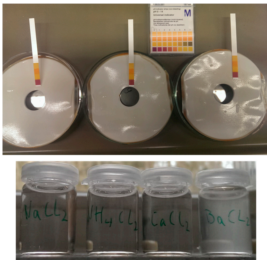
Figure 16. Acidic liquid on SILM envelopes (top) proven to contain \text{SO}_4^{2-} (white turbidity ( \text{BaSO}_4 ) in \text{BaCl}_2 ) (bottom).
