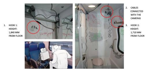
Fig. 5. Impression of the context and installation of cameras.
