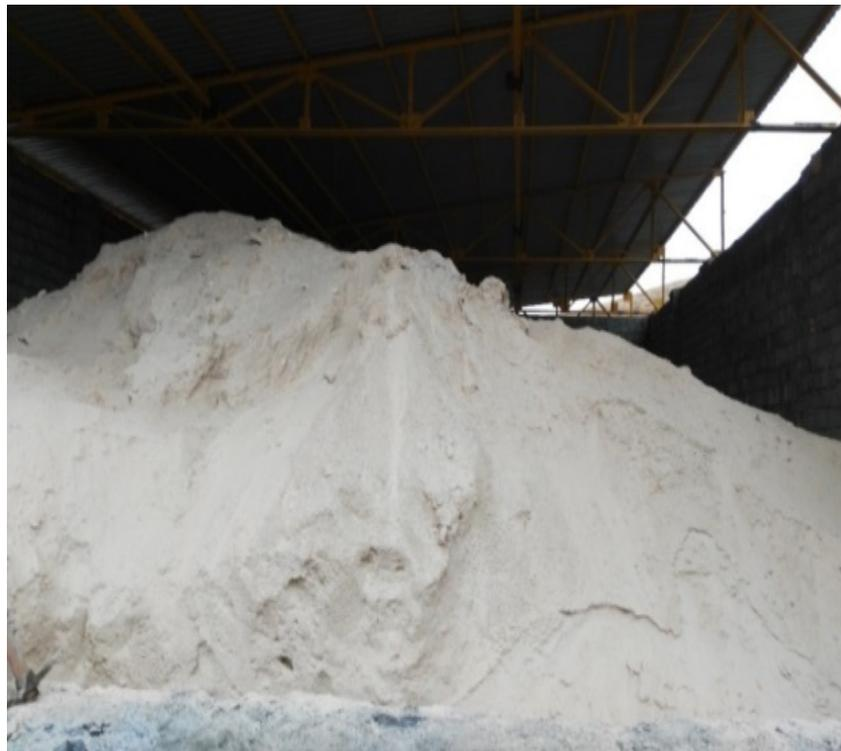
**Figure 1.** Silica stone waste (SSW) powder depot before the sieve.
