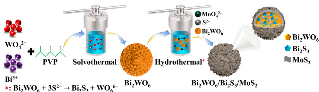
Scheme 1. Schematic diagram of preparing \text{Bi}_2\text{WO}_6/\text{Bi}_2\text{S}_3/\text{MoS}_2 heterojunction ternary composites.
