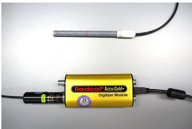
FIG. 1. A 10-cm ionization chamber and a digitizer module for CTDI measurement.
