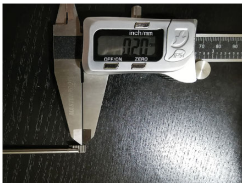
Figure A1. On the tip of our custom-designed graft-tunnel motion measurement device, each black block is 0.2 mm in width, as validated by a digital Vernier caliper (Masterproof).
