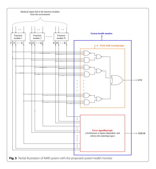
N-input NOR gates and AND gates in the first level, K numbers of K-input NOR gates in the second level, and a final K-input OR gate are required to realize the proposed fault warning logic. The gates present at any logic level may be optimally decomposed taking into account the fan-in restrictions of a digital cell library.
