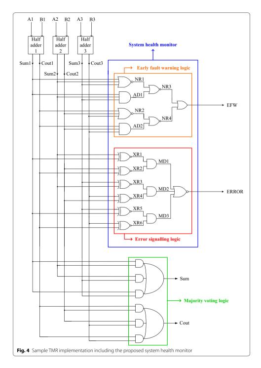
• No function module fault: Let us assume that half adders 1, 2 and 3 are fault-free. Hence the respective outputs of the half adders are equivalent, i.e. Sum1 = Sum2 = Sum3 and Cout1 = Cout2 = Cout3. Given this, NR1 = NR2 = 1/0 and AD1 = AD2 = 0/1 respectively. As a result, NR3 = NR4 = 0, which leads to EFW = 0. Also, XR1 up to XR6 would equate to 1, and hence MD1 = MD2 = MD3 = 1, resulting in ERROR = 0. Thus, EFW = ERROR = 0 which reflects the perfect healthy state of the TMR system.
