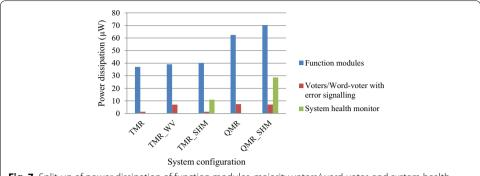
**Fig. 7** Split-up of power dissipation of function modules, majority voters/word-voter, and system health monitor (if any) corresponding to various TMR and QMR systems
