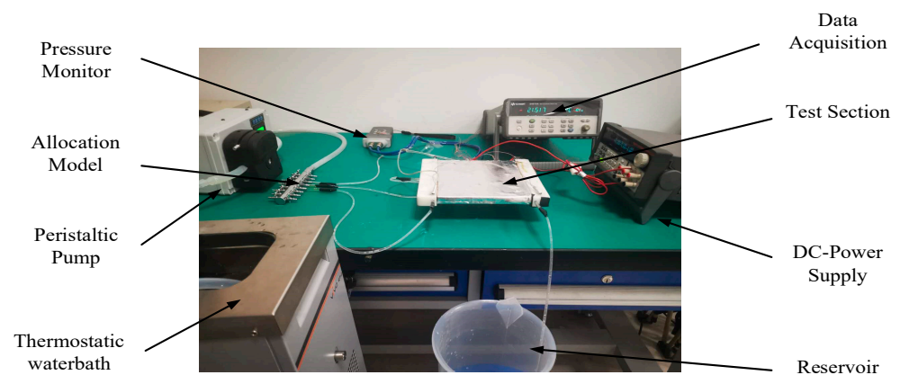
Figure 20. Testing apparatus for the performance evaluation.
