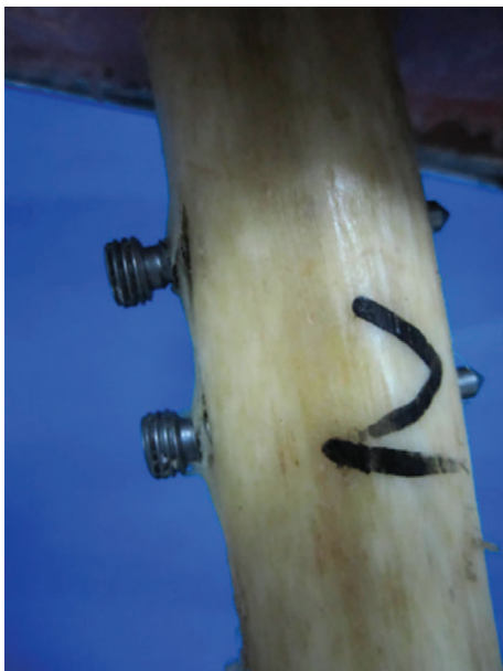
Fig. 6 The cortical bone around the proximal screw cap of the retrograde intramedullary nail was cleft under cyclic loading in 1 case.
