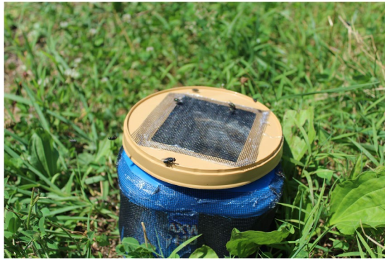
Figure 4. Holding container for aged chicken liver bait used to attract blow flies. The sides of the container, as well as the lid, have been cut open and covered with mesh. This aerates the container allowing for attractive volatile cues to disseminate into the surrounding environment while preventing the flies from landing on the bait itself.
