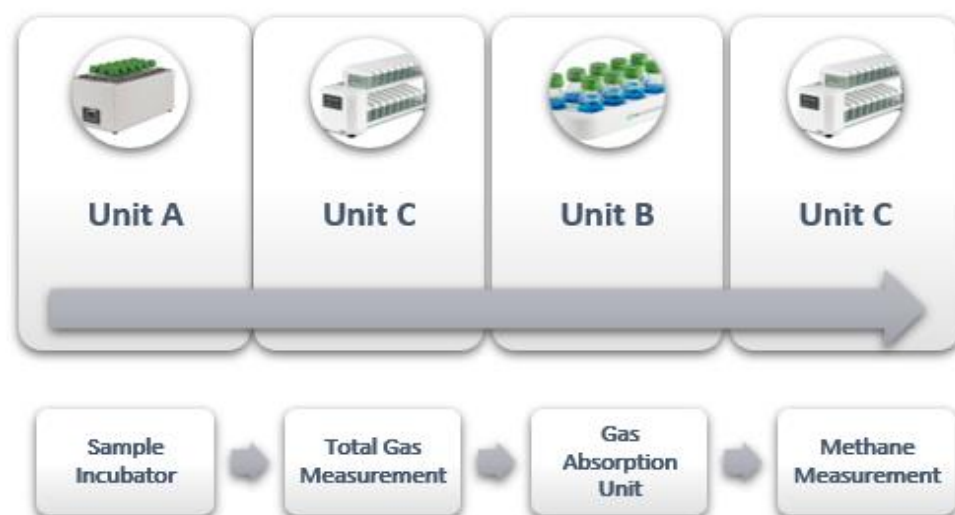
Figure 3. Workflow of the gas in the Gas Endeavour System (adopted from [46]).
