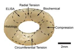
**Figure 2. Construct division for histological, biochemical, ELISA, and biomechanical assessments.** For biochemical, ELISA, and compressive testing 2 mm punches were removed from the construct. Tensile specimens were prepared by fashioning dumbbell shaped portions of the construct in the appropriate direction for circumferential and radial testing. After obtaining the above specimens, a sufficient portion was available for histological assessment. doi:10.1371/journal.pone.0027857.g002
