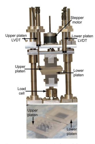
**Figure 1. Tension-compression stimulator and platens.** (Upper) Stimulation apparatus with relevant components labeled. (Lower) Rapid prototyped stimulation platens with upper platen possessing a curved surface to mate with the upper surface of meniscal constructs. doi:10.1371/journal.pone.0027857.g001
