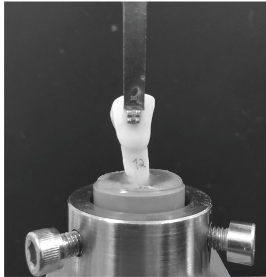
FIGURE 1: Specimen block mounted in the universal test machine.
