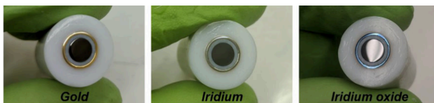
Figure 12. RRDE: Photographs showing an RRDE with gold disk and ring (left), after Ir metal deposition on the ring (middle), and after conversion to IrOx (right). Reprinted from ref 73. Copyright 2022 American Chemical Society.
