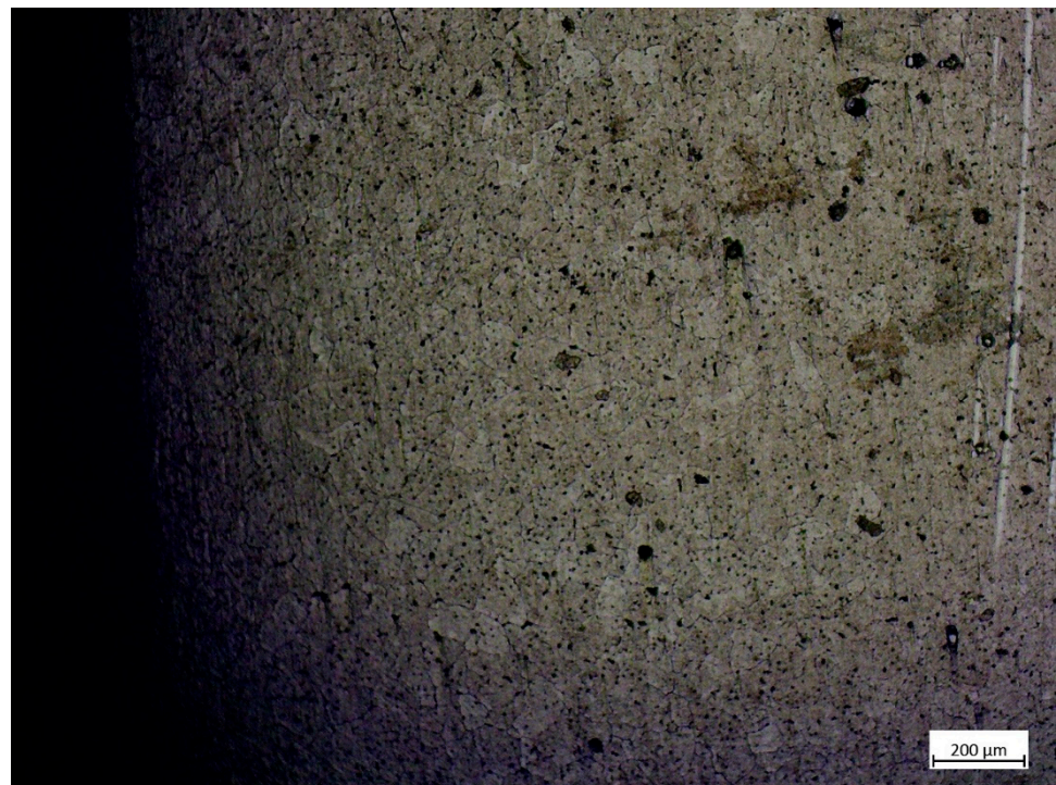
Figure 13. Etched metallography results of the base material using 50\times magnification.
