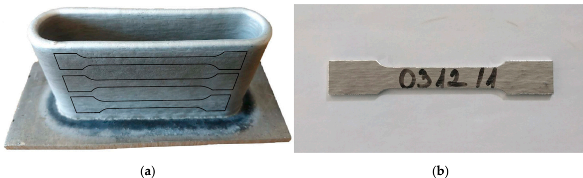
Figure 3. Production of stress test specimens perpendicularly to the weld direction: (a) location of specimen on the print; (b) machined specimen.
