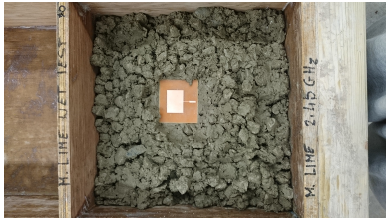
Figure 4. Smart sensor is embedded in the concrete block for moisture detection.
