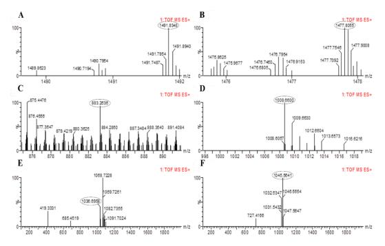
**Figure 5.** LC-MS chromatogram of methanolic extracts of *B. altitudinis* HNH7. (**A**,**B**) = Fengycin; (**C**) = Bacillibactin; (**D**,**E**)= Surfactin and (**F**) = Bacillomycin.
