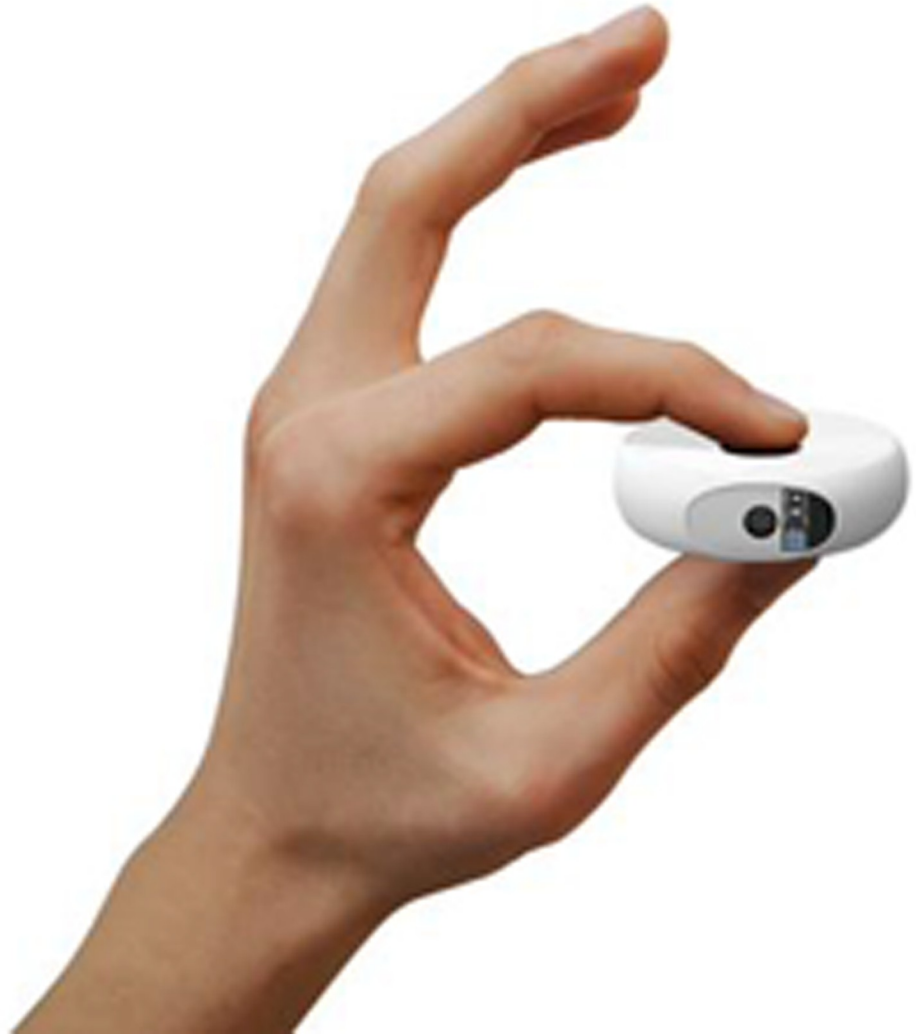
Fig 1. Scanadu scout device. The Scanadu Scout device records physiological measurements when held to the forehead. (Source: Scanadu with permission).
