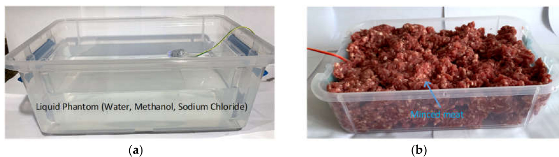
Figure 12. Measurement setup to test the transmission rate of the proposed capsule in: (a) liquid phantom; (b) minced meat.
