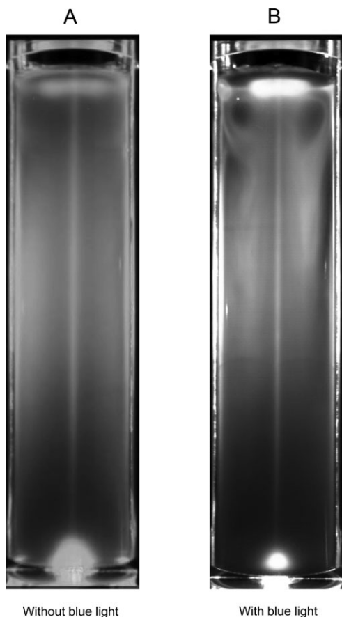
Fig. 2. Phototaxis is required for vortical distribution. Time-averaged image of motile cells (wt) with (A) or without (B) blue light for phototaxis (cell concentration C=1\times 10^6 cells/ml, bubble flow rate Q=100 \mu\text{l}/\text{min} , diameter D=40 mm). Inhomogeneous distributions were created with or without phototaxis, although this was stronger with phototaxis. However, vortical distribution was only observed with phototaxis. The images are averaged over 10 min for three independent experiments.
