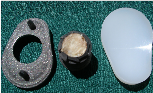
Figure 7a: Retrieval specimen, intact cage screw with excellent bone in-growth in central core without evidence of bone on-growth to the glenoid component
