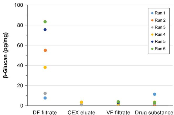
**FIGURE 3**  $\beta$ -Glucan content measured in different in-process samples for mAb 4. Data were obtained from six runs at pilot scale (2000 L)
