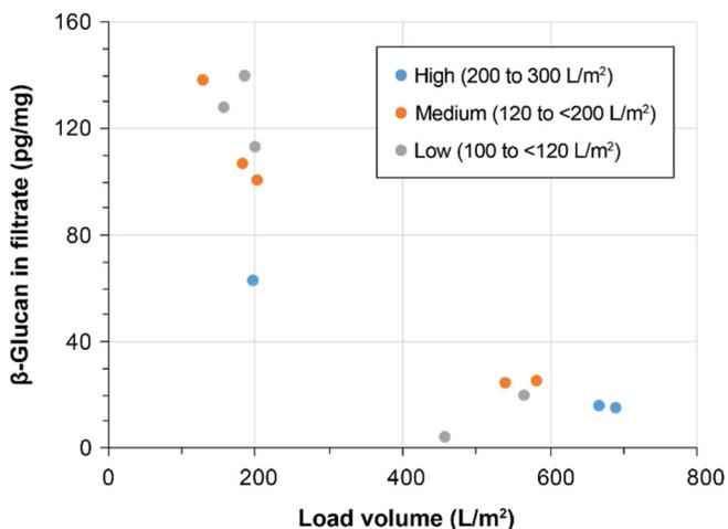
**FIGURE 2**  $\beta$ -Glucan content measured in the depth-filtration filtrate for mAb 5. Data were obtained from laboratory scale production (80 or 200 L) using a Zeta Plus 60Z B05A depth filter. Before filtration of the neutralized Protein A eluate, the filter was flushed with 100–300 L/m<sup>2</sup> water
