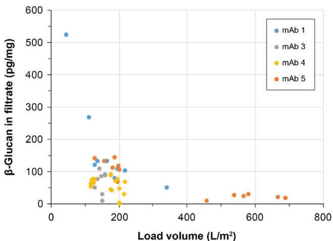
**FIGURE 1**  $\beta$ -Glucan content measured in the depth-filtration filtrate for four different mAbs at different load volumes. Data were obtained from different production scales. Zeta Plus 60Z B05A depth filter was used for all four mAbs
